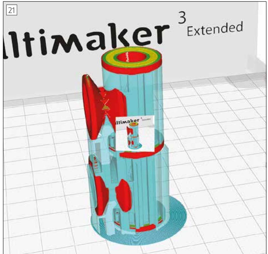
Preparing a print of a capstan wrap in Cura. Material shown blue is the support structure with a brim to provide good attachment to the build plate.
