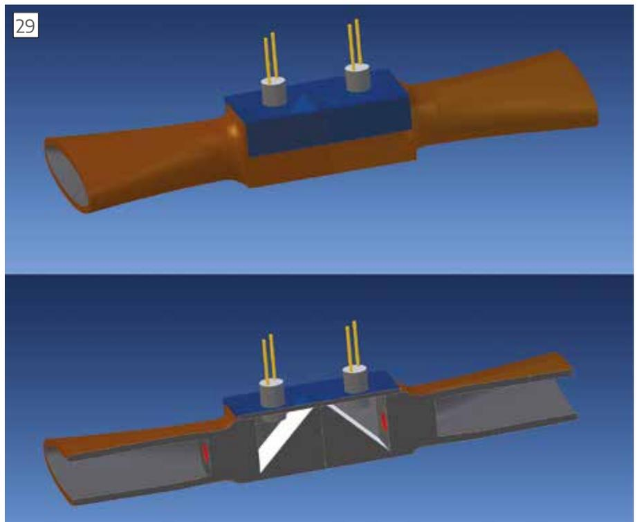
Alibre model of the Optical Horizon Sensor with a section through the assembly. Light entering the cone excites fluorescence in the rod which reflects off a screen viewed by the LDR.
