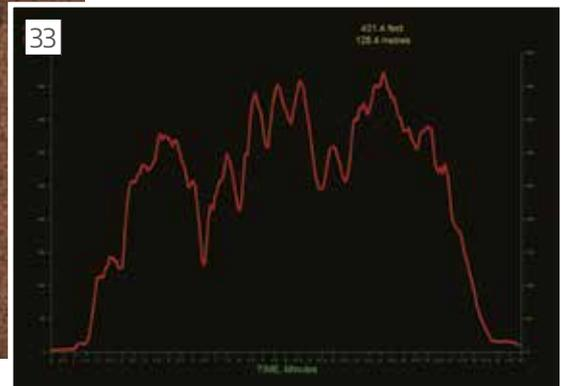
An example of the altimeter log with the peak altitude identified in feet and metres.
