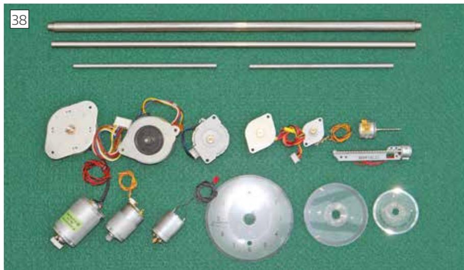
A small selection of parts salvaged from redundant inkjet printers. These include stepper and servo motors, precision shafting and rotary encoders.
