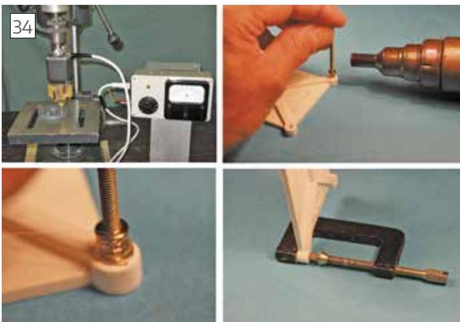
Various methods for staking threaded inserts. Clockwise from top left: With heat staking machine (MEW 225-227); Hot air gun and studding; Using glue and heat; Simply forcing in with a vice or arbor press.
