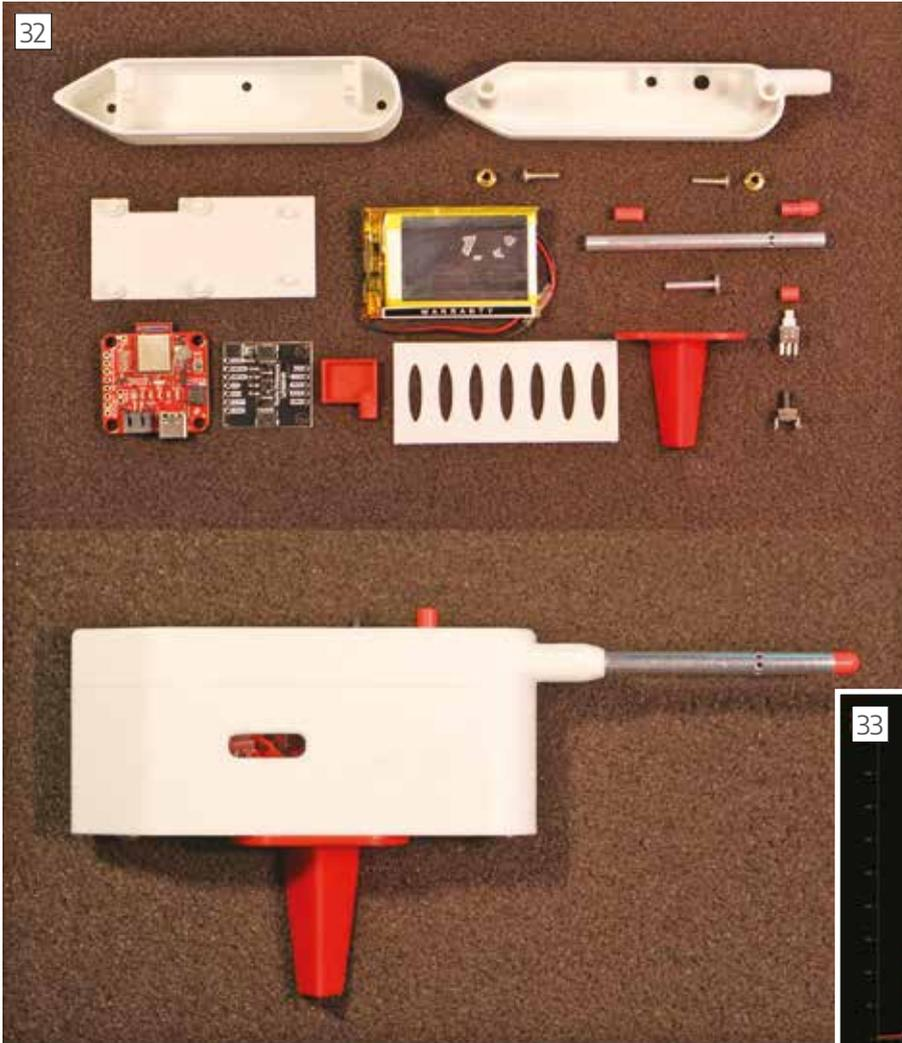
Components of the altimeter and the assembled unit ready to fly.
