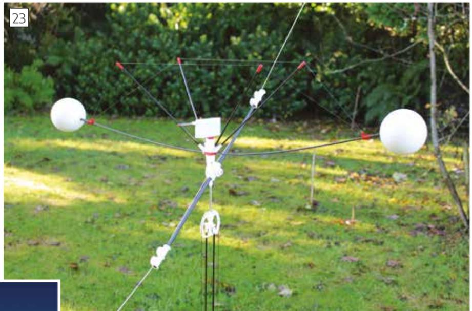
*Passive ball stabiliser, braced to prevent aerodynamic flutter.*
