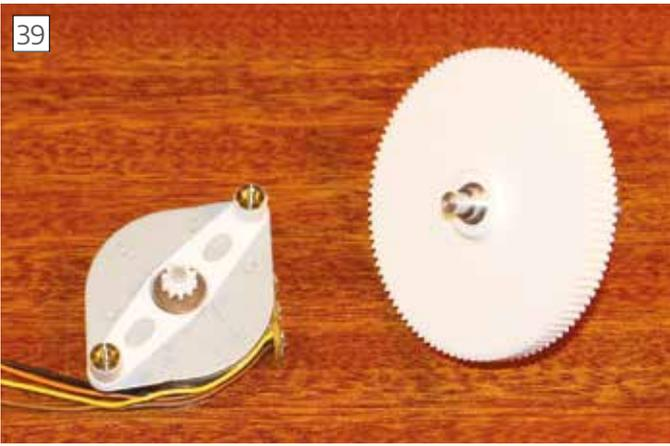
3D printed involute gears that transmit drive from the motor to the output shaft of the PanGimbal. These have provided negligible backlash and undetectable wear.
