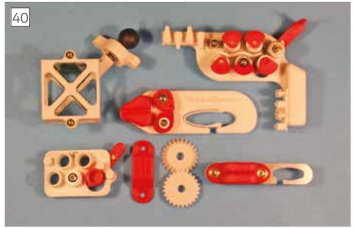
Other gadgets produced using 3D printing that play an important part in my KAP activity. These include cleats, a camera mount and two concepts for a line payout.
