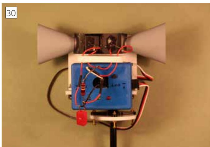
Rig to evaluate the LDR-based Optical Horizon Sensor.
