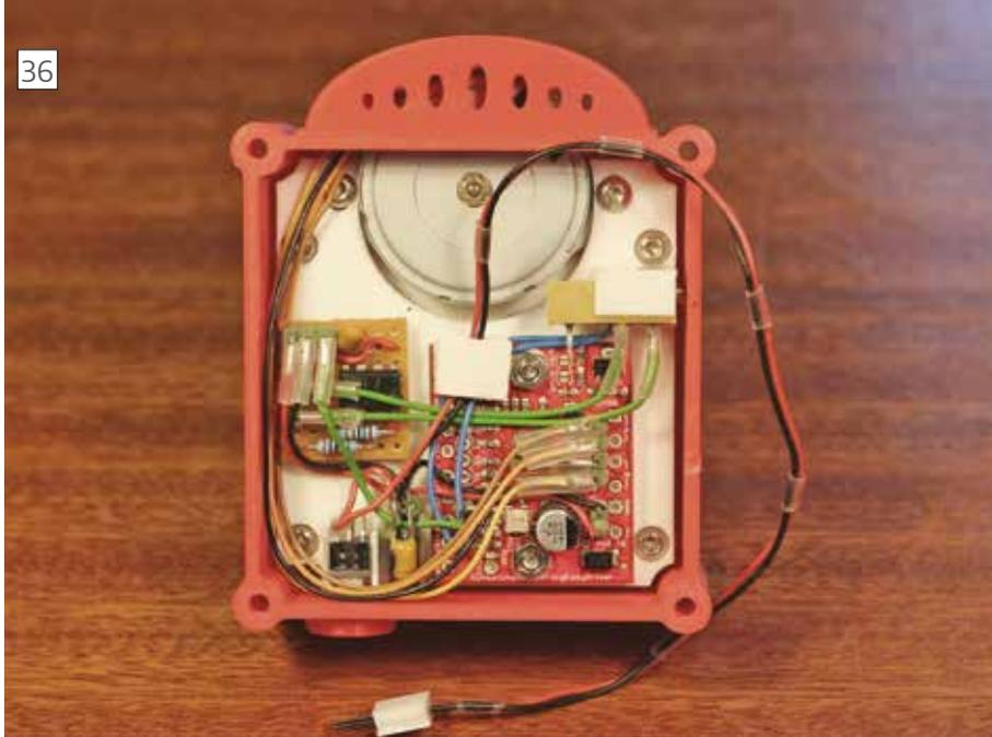
Internal view of the PanGimbal showing the stepper motor, BigEasy Driver, pulse generator and regulator.
