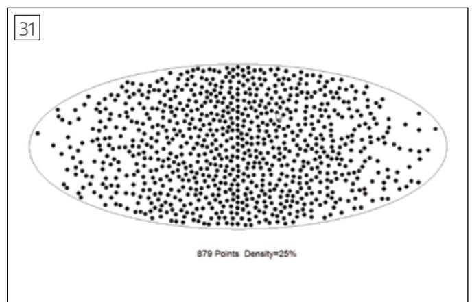
Example of a shadow mask for the optical horizon sensor made by printing a graduated pattern of dots on transparent acrylic film.
