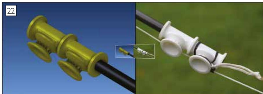
Alibre model and close-up of one of the printed capstan wraps. The black rubber band is added for security in case the line goes slack when flying.
