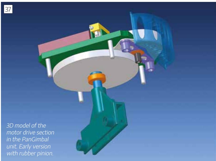
3D model of the motor drive section in the PanGimbal unit. Early version with rubber pinion.
