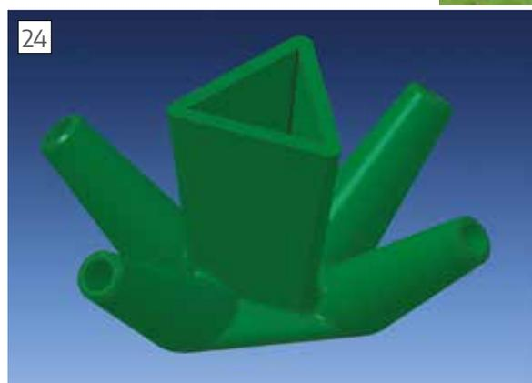
*Boss at the centre of the ball stabiliser with 4 diverging pillars made by projecting from the faces of an extruded hexagon in Alibre.*
