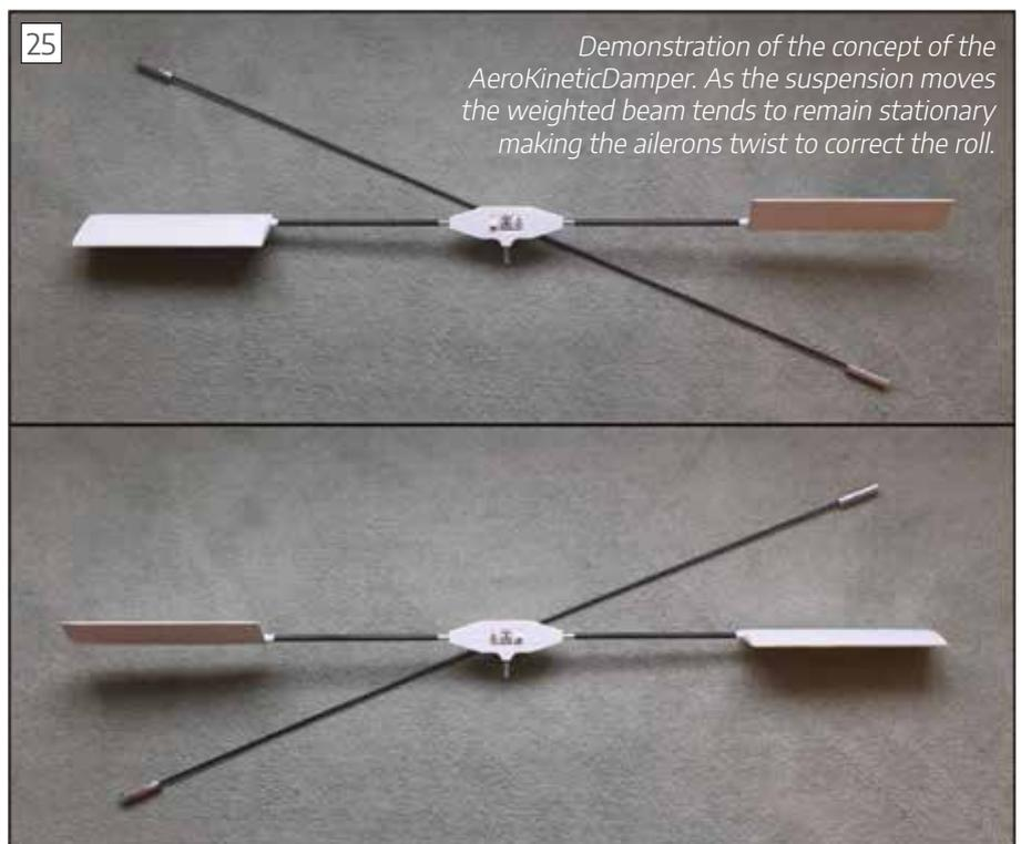
*Demonstration of the concept of the AeroKineticDamper. As the suspension moves the weighted beam tends to remain stationary making the ailerons twist to correct the roll.*
