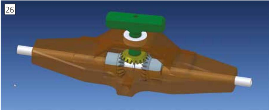
Alibre model of the differential gearbox at the heart of the AeroKineticDamper.
