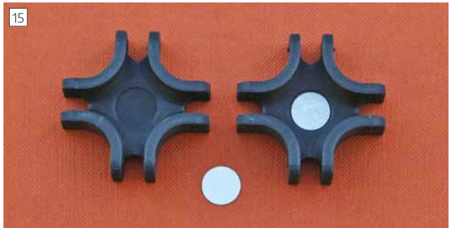
Carbon-nylon composite spider hub printed by Additive-X in a Markforged machine. An aluminium disc is bonded to the centre to act as a hard bearing plate for the ends of the spider arms.
