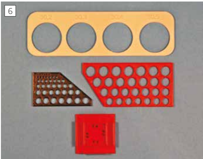
6 A selection of gauges printed to determine optimum sizes to incorporate in particular design models.
