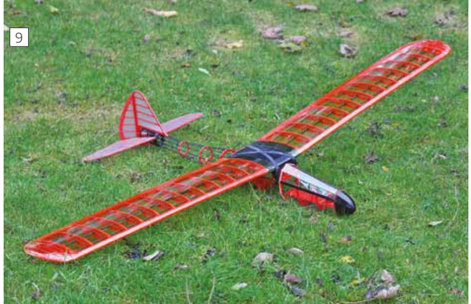
Model aircraft built using printed parts and carbon fibre.
