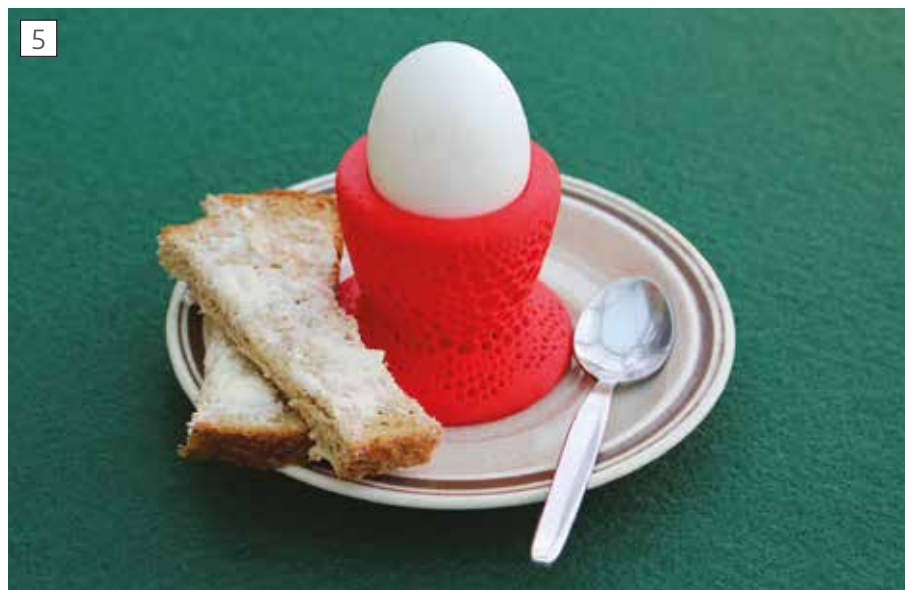
Egg cup designed using Alibre, latticed with Meshmixer, printed in an Ultimaker 3.
