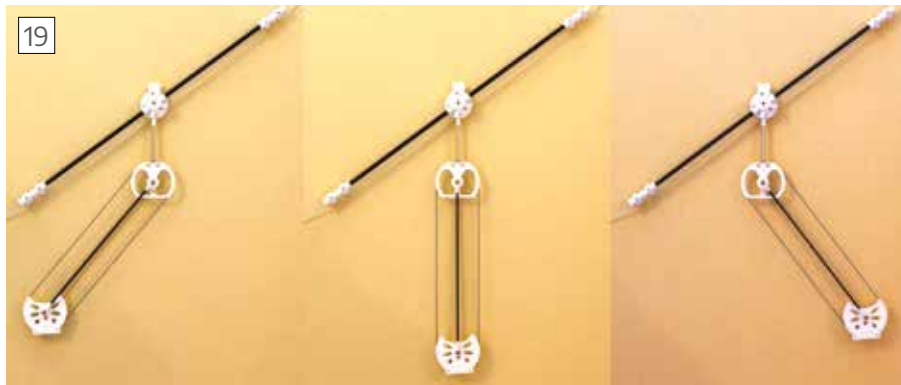
Sequence of images showing how the geometry of the aeronaut suspension maintains the camera (to be attached at the bottom) at a constant angle relative to the kite line.
