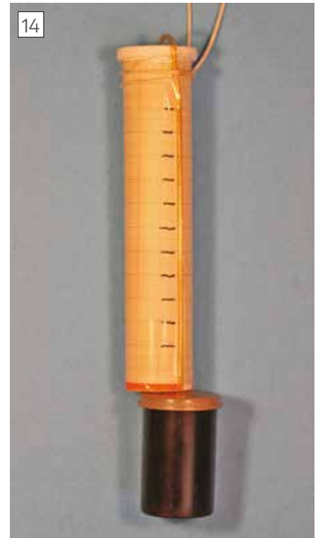
Replica of the capillary-bubbling altimeter. As the unit ascends air expands from the larger reservoir through the narrow tube and bubbles into water contained in the smaller reservoir. During the descent water is drawn up the tube to a level that records the peak altitude. Patent Still Pending.
