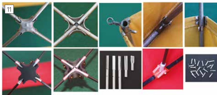
Top: Details in the frame of the Gibson Girl kite. Bottom: details in the frame of the Gibson Boy.
