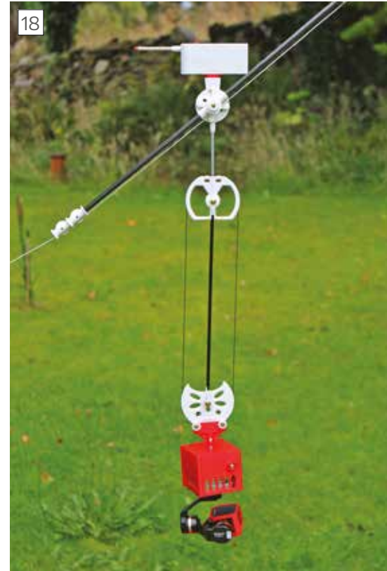
New type of Aeronaut suspension made of 3D printed parts and carbon fibre tube. The altimeter is fitted into the TriTaper socket at top, while the PanGimal unit and camera is attached at the bottom.
